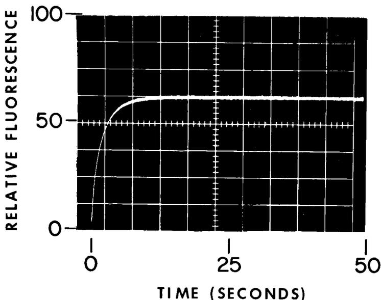
*Figure 2:* Oscilloscope photograph of the reaction of fluorescamine with alanine at pH 9.0 in the Aminco-Morrow stopped-flow fluorometer.
