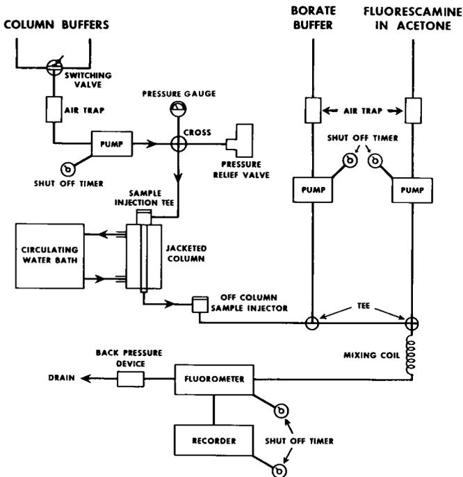
Figure 3: Schematic illustration of the flow system for automated assay with fluorescamine. Milton Roy minipumps were used for the column as well as for the 0.2 M sodium borate, pH 9.7 and 15 mg% solution of fluorescamine in acetone. A Beckman recorder and an Aminco filter fluorometer were employed.
