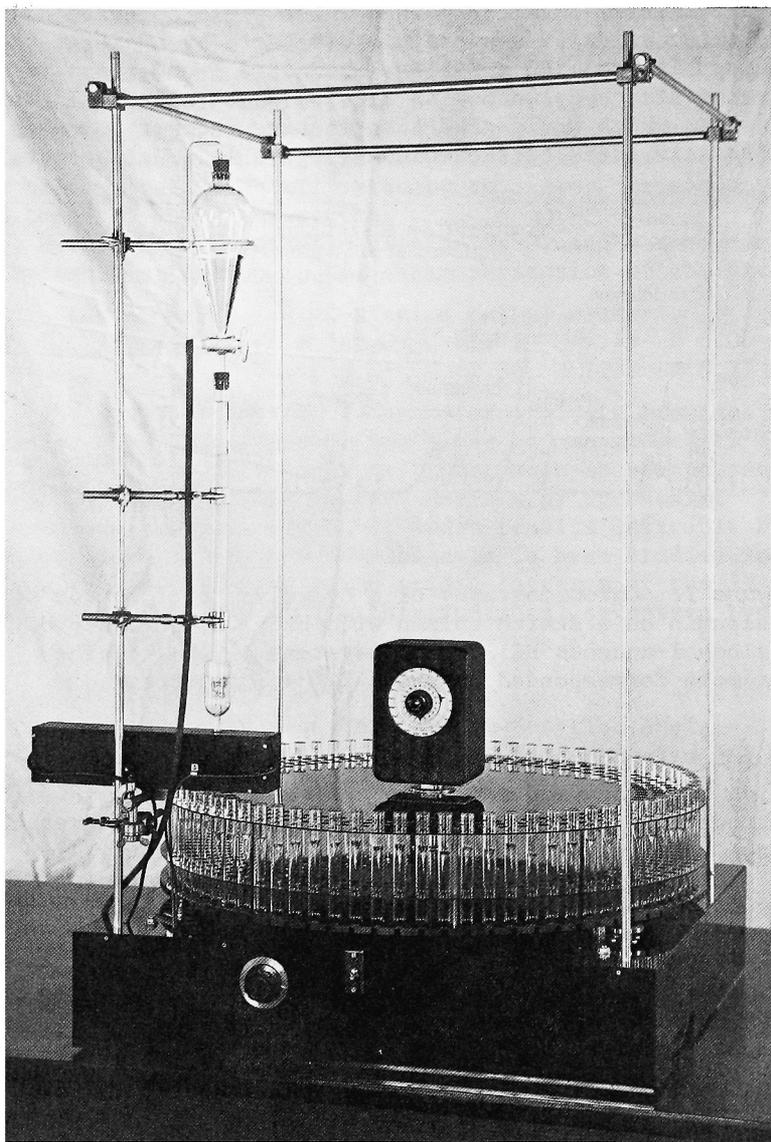
*Figure 2:* Automatic fraction collector for chromatographic analysis with volume control by the counting of drops (1948).<sup>8</sup>
